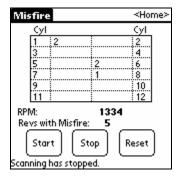
Press the Start button to start scanning. The chart will be updated as misfires are detected. In the example above, cylinders 1 & 6 have had 2 misfires, and cylinder 8 has had one. You can see the current RPM and how many rev's have had misfires below the chart. The status is at the very bottom. The Reset button will set all misfire counts back to zero & clear the chart, and the Stop button will suspend scanning.
